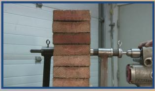
The Ferreras Drill Alignment Tool is a tool used for guiding a drill through piling foundations for the installation of column caps. The device clamps to the piling on both sides of the column cap and aligns the drill bit properly to efficiently bore through pilings. A true hole is made to perfectly reach the opposite eye bolt hole in the column cap.
